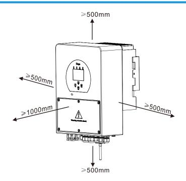
For proper air circulation to dissipate heat, allow a clearance of approx. 50cm to the side and approx. 50cm above and below the unit. And 100cm to the front.
