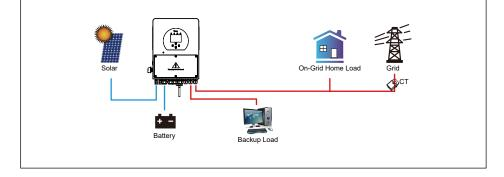
**Solar Sell:** "Solar sell" is for Zero export to load or Zero export to CT: when this item is active, the surplus energy can be sold back to grid. When it is active, PV Power source priority usage is as follows: load consumption and charge battery and feed into grid.
