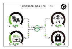
1. The icon in the center of the home screen indicates that the system is Normal operation. If it turns into "comm./FXX", it means the inverter has communication errors or other errors, the error message will display under this icon(FXX errors, detail error info can be viewed in the System Alarms menu).
