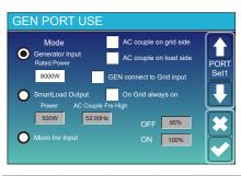
Generator input rated power: allowed Max. power from diesel generator.
