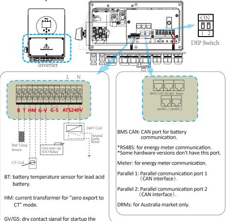
When the "GEN signal" is active, the open contact (GV/GS) will switch on (no voltage output). If the "Signal ISLAND MODE" is ticked, the GS port will be the dry contact signal for startup the diesel generator. If "Signal ISLAND MODE" is not ticked, the GV port will be the dry contact signal for startup the diesel generator.
