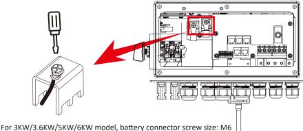
4. In case of children touch or insects go into the inverter, Please make sure the inverter connector is fasten to waterproof position by twist it clockwise.
