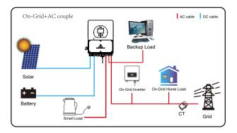
The 1st priority power of the system is always the PV power, then 2nd and 3rd priority power will be the battery bank or grid according to the settings. The last power backup will be the Generator if it is available.
